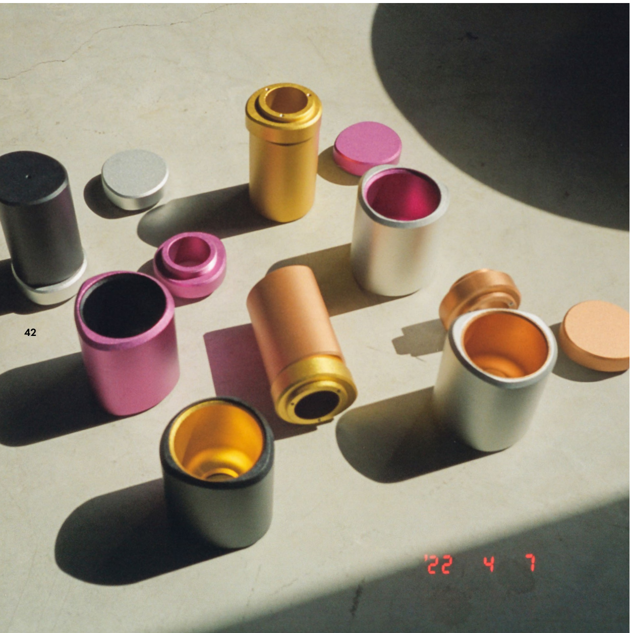
Colour testing for the cylindrical sections that are machined from solid billet aluminum in a hard anodized finish.
